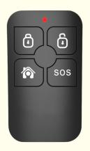
The Milan Vortex Keyfob is used to trigger four different actions. One of the buttons can be used to trigger a panic alarm that can alert others using MyMilan app notifications. The other buttons can be used to activate convenience features such as MyMilan scenes or turning off all lights when leaving home.
